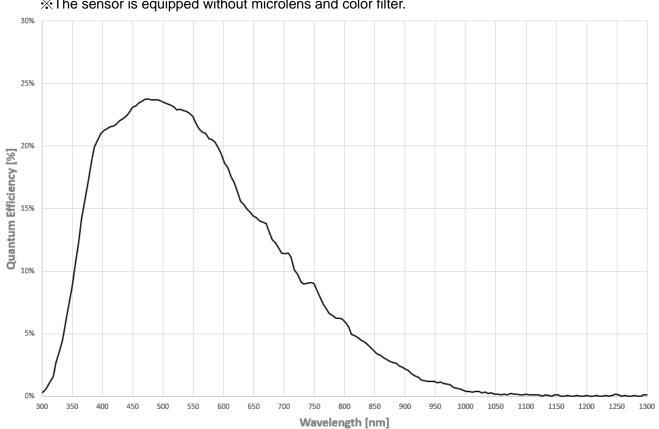
$\ensuremath{\ensuremath{\mathbb{X}}}$  The sensor is equipped without microlens and color filter.
