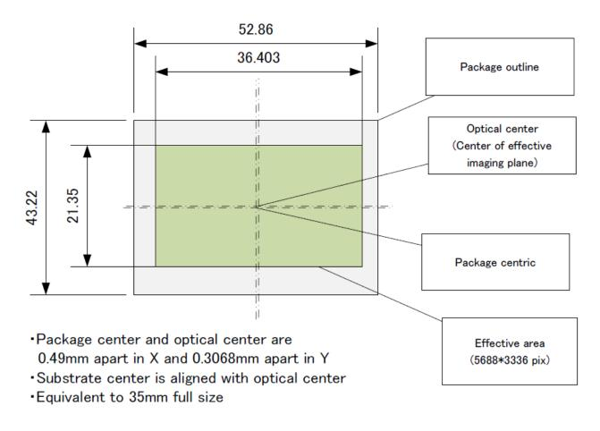
H=6.4[µm] \* 5688 = 36403.2[µm] V=6.4[µm] \* 3336 = 21350.4[µm]
