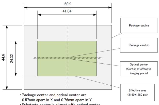
·Substrate center is aligned with optical center
