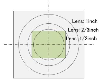
\*The ratios of sense. One cangestary to foul one in the above matrices are as follows:  $1/2 \text{ inch} = \phi 8 \text{mm}, 2/3 \text{ inch} = \phi 11 \text{mm}, 1 \text{ inch} = 15.8 \text{mm}.$
