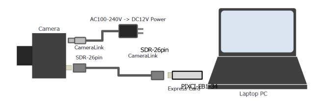
For the connector of this camera is SDR-26pin, please use the supported cable.
