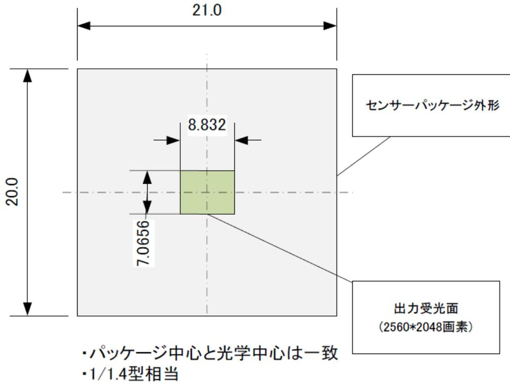
$$H = 3.45[\mu\text{m}] * 2560 = 8832[\mu\text{m}]$$
